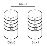
If a drive failure occurs, read and write operations are directed to the remaining drive. A replacement drive can then be rebuilt using the data from the remaining drive.
